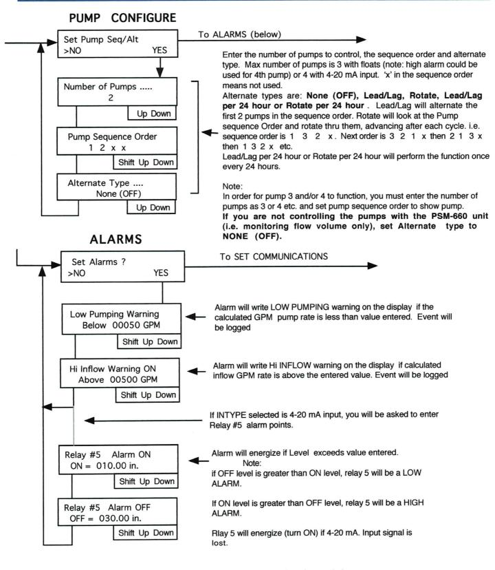
NOTE: If High or Low alarm is sounded, press any button on the front panel to silence the alarm (deenergize relay #4 and/or relay #5).
